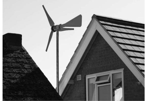
**This small rooftop wind system is located too close to rooftops, other buildings and trees; all of these cause turbulence that reduces the effectiveness and performance of the turbine..**
